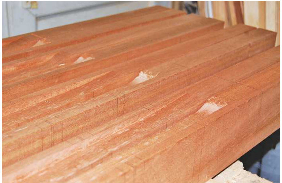
▲ Pic 5 Here are the stopped rebates on the middle rails
